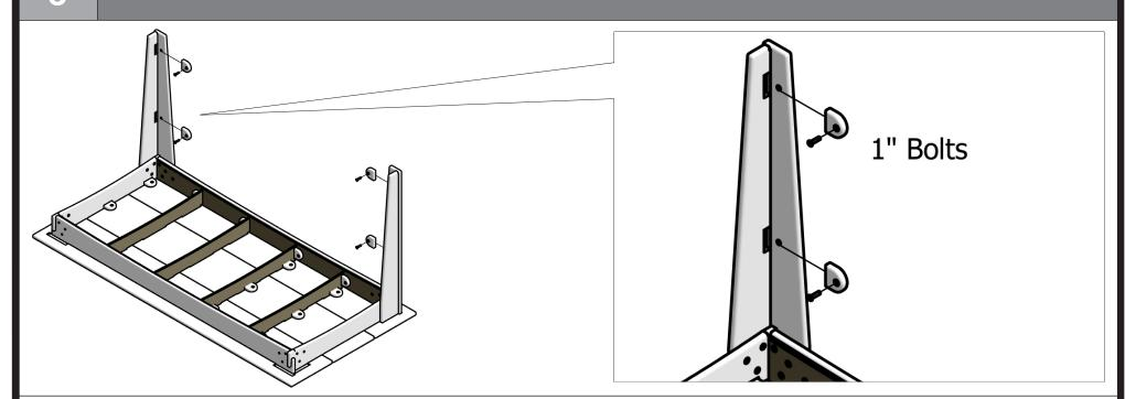
Fit Lock Blocks G into the Left & Right Legs B pocket cut outs. Place 1" bolts through the Blocks G into the Left & Right Leg B threaded holes and finger tighten.
