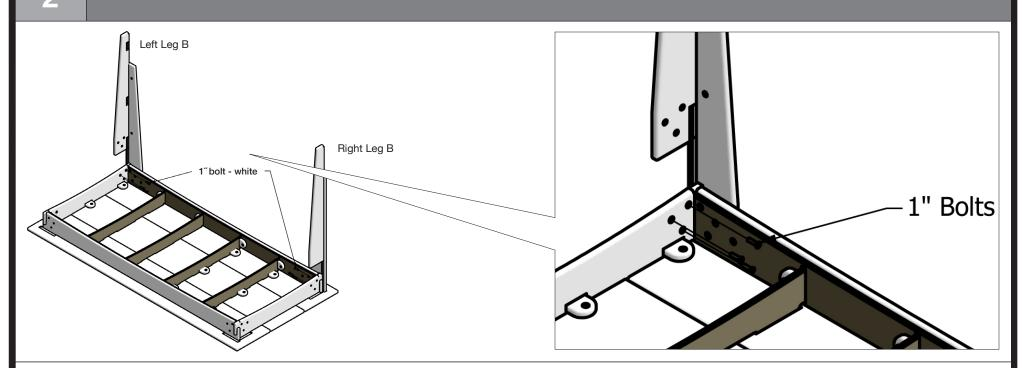
Fit the Left & Right Legs B into the groove track cut out of the Left & Right Legs A and slide it down into the Top pocket cut outs. Insert 1" (white) bolts through the side brace holes into the Legs threaded holes and finger tighten.
