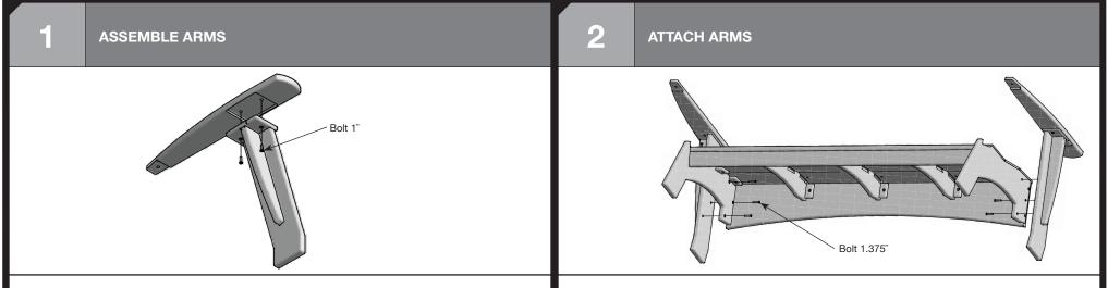
Align holes of arm rest with arm support holes. Insert 1" bolts through
