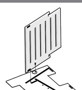
\*Please read **Assembly Tips** before beginning assembly. Fit Back edge into Left Side groove track cut out with the pocket cut out in the Back facing the threaded insert in the Left Side. Place Block G into Back pocket cut out and insert bolt through the block into Left Side threaded hole and finger tighten.
