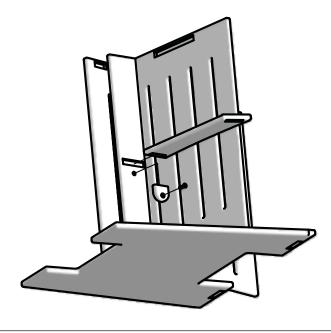
Fit Mid brace straight edge into Back Brace pocket cut out. Place Block G into Mid Brace pocket cut out and insert bolt through the block into the Back Brace and finger tighten.
