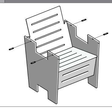
Attach right side using steps 1,2, & 4. Fit Micro Double Blocks through the holes in the Left and Right sides so each block has a hole exposed on each side.
