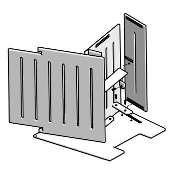
Fit Face Plate short edge into Left Side pocket cut out and fit Mid Brace angled edge into the Face Plate pocket cut out. Place Block G into Mid Brace pocket cut out and insert bolt through the block into the Face Plate and finger tighten. Place Block B into Face Plate pocket cut out and insert bolts through the block into the Left Side and finger tighten.
