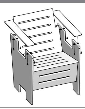
Fit Left and Right Arms cut outs over Left and Right Sides with Micro Double Blocks. Insert 1/2 "Round Head Bolts through the blocks into the Arms and finger tighten.
