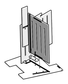
Fit Seat edge into Left Side groove track cut out with the Seat's groove track cut out towards the Back. Place Block B into Seat pocket cut out and insert bolts through the block into Left Side threaded holes and finger tighten.
